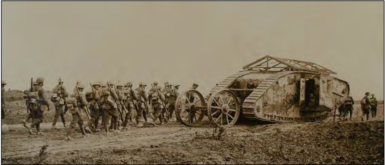
A tank on the Western Front. The cage on top was designed to help grenades bounce off.
